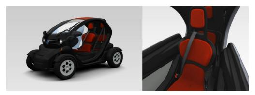
The Renault Twizy with Autoliv's new 2+3 point seatbelt concept. The regular 3-point belt on the Twizy's left side is supplemented with a 2-point belt over the driver's right shoulder.
